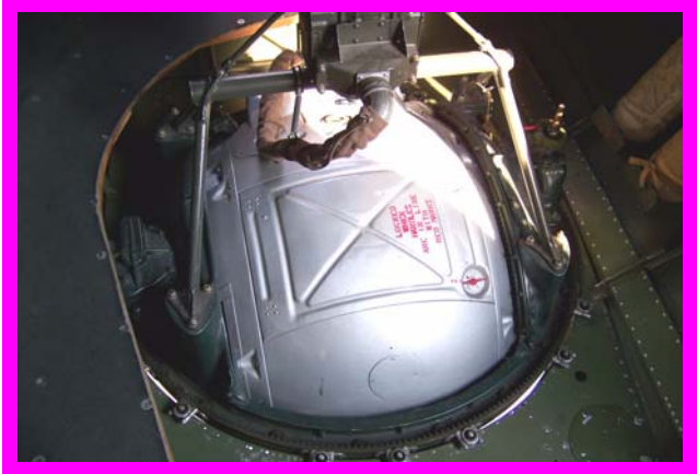
You had to be very small to access the ball turret (from outside only) The ball turret from inside the aircraft
