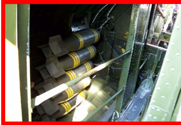
The Bomb rack for a total of 20, 500 pound bombs
