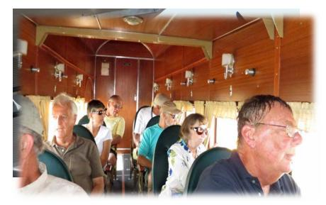
There are 18 available passenger seats in this beautiful main cabin, and all were full for our flight. Known as the "Tin Goose", due to its corrugated metal surface, our ship was powered by three Pratt & Whitney Wasp, 9 cylinder radial engines, each producing 420 horsepower. While this airplane has a top speed of 150 MPH, its normal cruise is 90, or just about the same as my little home built.
