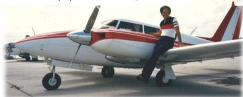
one very pretty package. With a cruise speed of almost 200 MPH it would burn far less than 15 gallons per hour at economy cruise. It could get me up to 18 thousand feet and it would carry all of my testing equipment, 300 bulky pounds worth, after I removed 3 of its 6 seats. It was a very stable instrument platform and allowed me to cover a wide portion of the US in my non-destructive testing business. My particular twin-Comanche had
